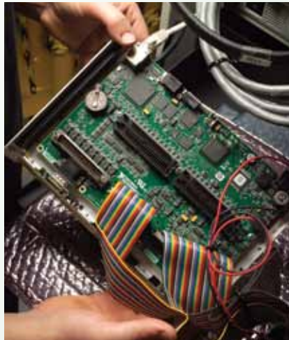
The EcoCar's supervisory control system will be programmed onto this sbRIO hardware from National Instruments.
